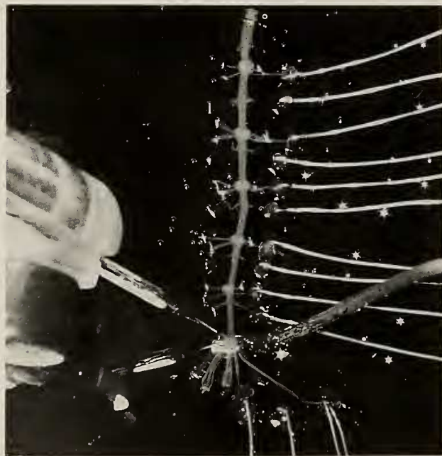
FIG. 1. The picture of experimental arrangement with extracellular and intracellular electrodes. The abdominal nerve cord was dissected out from the 1st to terminal abdominal (A6) ganglion. The motor activities of the uropod and abdominal postural system were monitored from relevant motor nerve root with pin electrodes. Electrical stimulation was delivered to the 2nd root afferents of the terminal abdominal ganglion by the bipolar electrode. The intracellular recording and stimulation was made from the terminal abdominal ganglion.
